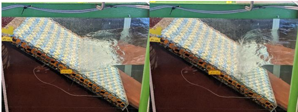
Figure 6. Coastalock 2D Physical model tests in TU Delft
