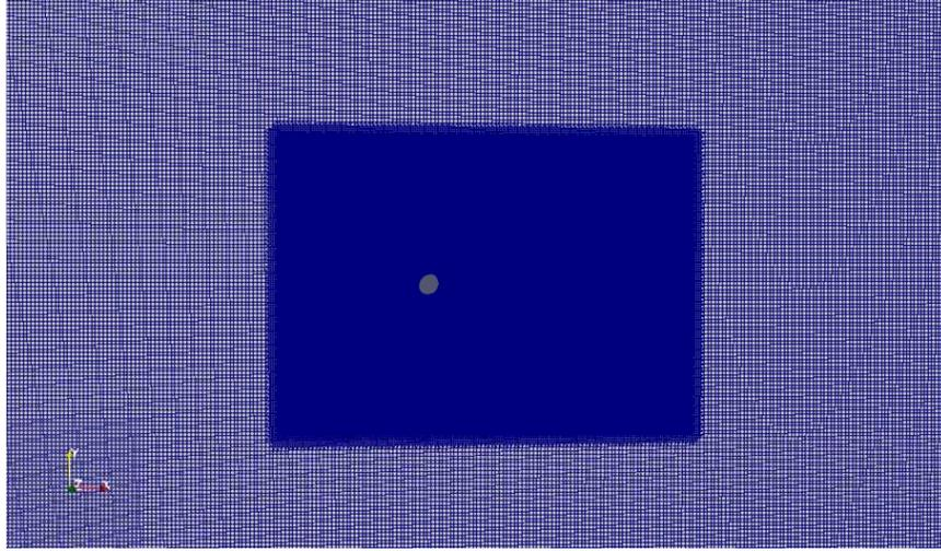
Figure 2. Mesh zones around the monopile foundation (gray) – horizontal view. (the visual mesh shift is coming from ParaView visualization)
