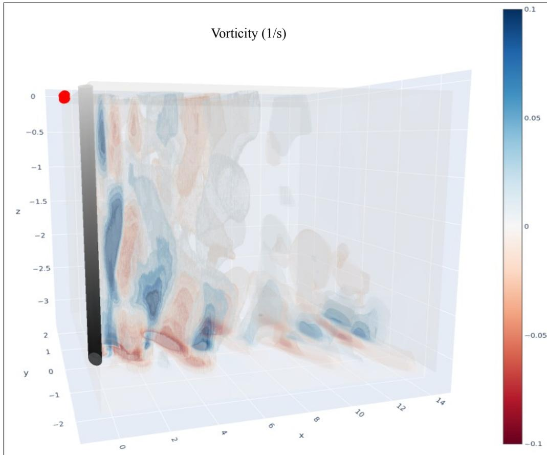
*Figure 5. 3D visualization ( $x$ =longitude,  $y$ =latitude,  $z$ =depth) near the monopile (black cylinder) of the magnitude vorticity with initial position of the particles dispersion at the surface (red dots).*
