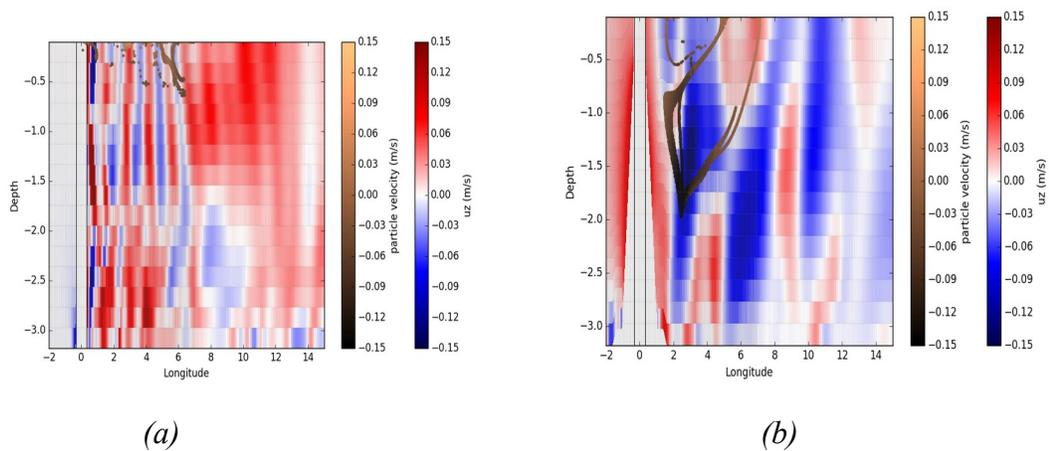
Figure 7. Vertical view ( $x$ - $z$  : in the latitude layer in the center of the pile) of vertical velocity with larval particles after 30s from release at the surface layer: (a) simulation with monopile structure (b) simulation with gravity base structure.
