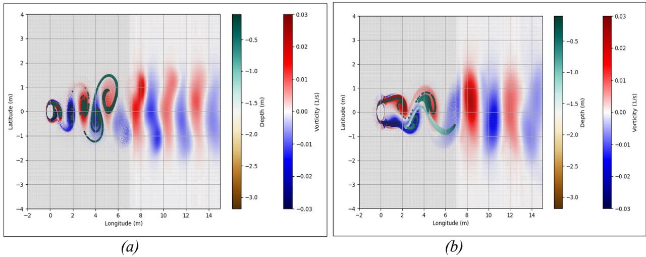
Figure 3. Horizontal view (lon-lat) for depth on the surface of vorticity magnitude with larval particles (dots colored by depth position) after 25s of release at the surface in front of the pile. (a) monopile structure and (b) gravity base structure.
