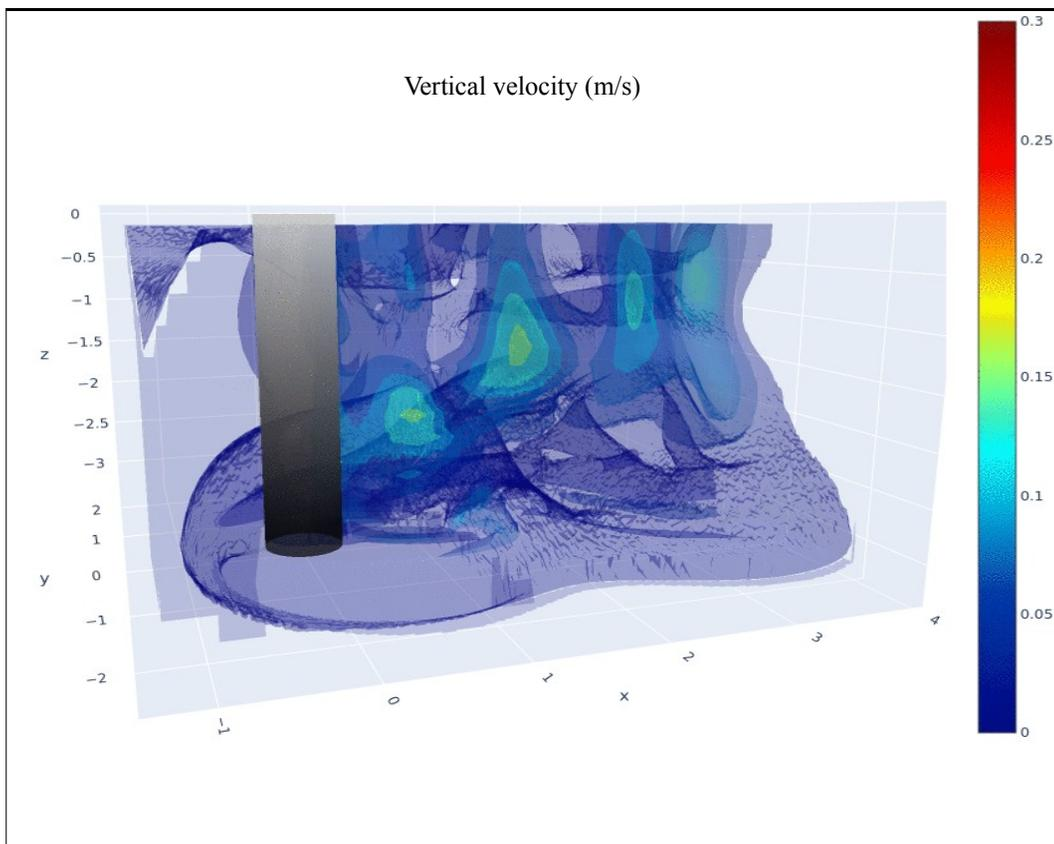
Figure 4. 3D visualization ( $x$ =longitude,  $y$ =latitude,  $z$ =depth) of the vertical velocity  $U_z$  close to the monopile.
