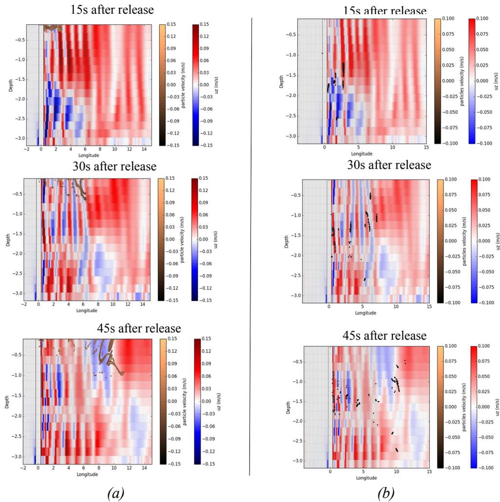
Figure 6. Vertical ( $x$ - $z$  : in the latitude layer in the center of the pile) of vertical velocity with larvae (dots colored by depth position): (a) released at the surface layer and (b) release at 2m under the surface layer.
